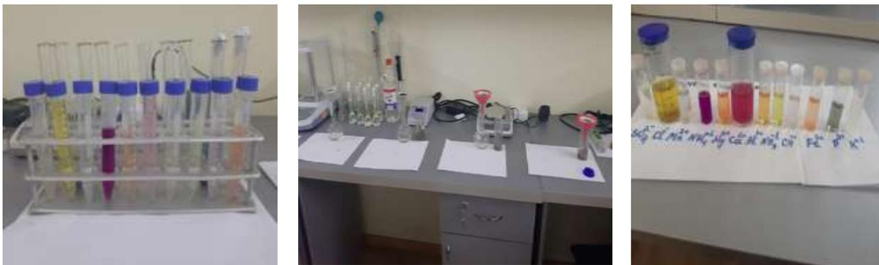
Figure 10. Analyzes with 14 parameters according to mineral content with Palintest soil kits 400 equipment
