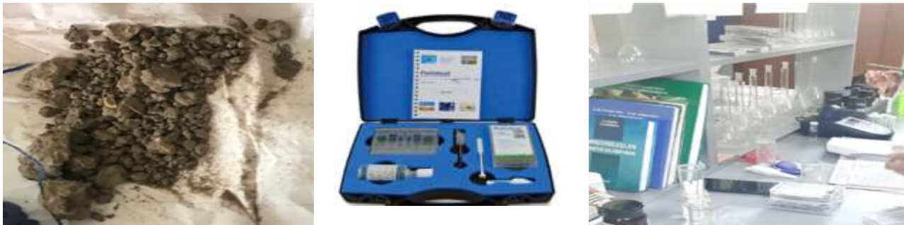
Figure 9. Analysis of a soil sample brought from the surrounding area of Zangilan district in the laboratory using Palintest Soil equipment in the Plant ecology laboratory of the institute
