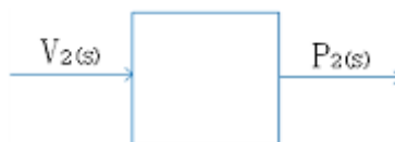
Figure 4. Black box for hydraulic energy circuit
